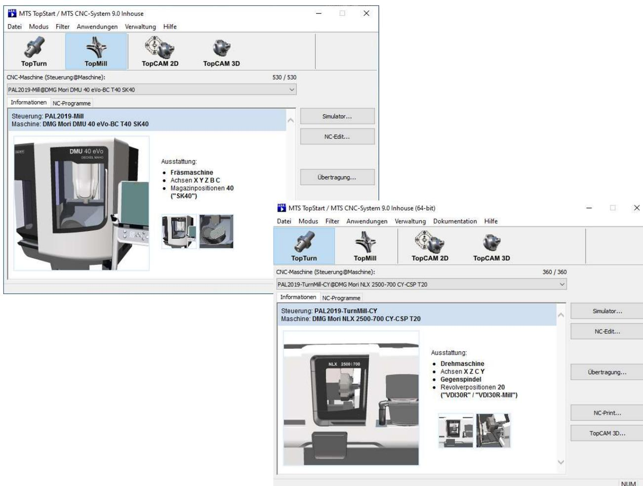
The screenshot shows two overlapping windows of the MTS TopStart software. The top window is titled "MTS TopStart / MTS CNC-System 9.0 Inhouse" and shows the "PAL2019-Mill" machine configuration. The bottom window is titled "MTS TopStart / MTS CNC-System 9.0 Inhouse (64-bit)" and shows the "PAL2019-TurnMill-CY" machine configuration. Both windows feature a menu bar, a toolbar with application icons, and a main content area with a 3D model of the machine and a list of equipment.
